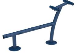
All Steel components are made from carbon steel, with a hot-dip galvanized surface according to ISO1461, and a powder coating corrosion class C3 according to ISO12944-2. Lead content for surfaces is below 90ppm, and below 100ppm for base material.
