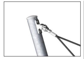
The swing hangers are made of stainless steel brackets and can move over two axis. The flange bearings are silicone enriched to make the suspension maintenance free. At the rope fixation there is a turnable anti twist functions that prevents winding up the ropes.
