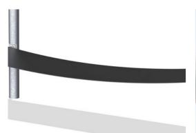
Membrane consisting of friction-proof rubberized material of conveyor belt quality with excellent UV resistance. Tested and compliant with REACH requirements for PAH. Embedded are two layers of galvanised steel wire armoring, making the membrane extremely hardwearing and vandalism resistant. Core and outer layers result in a total thickness of 10mm.
