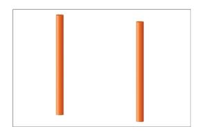
The Steel posts are made of Ø101,6x2,0mm pre-galvanized steel tube. The posts are powder coated, corrosion class C3 according to ISO12944-2.
