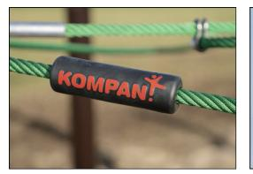
Ropes of UV-stabilized PES rope strands with inner steel cable reinforcement. The polyester yarn is made from +95% post-consumer materials and is inductively melted onto each strand. Colored steel components have a base of hot dip galvanization and a powder coated top finish. This provides an ultimate corrosion resistance in all climates around the world. Other steel surfaces are hot dip galvanized inside and outside with lead free zinc.
