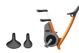
The saddle is made of a Polyurethane Rubber and has a steel insert plate which connects it to the aluminium saddle pin. The saddle can be adjusted to 13 different heights, using a stainless steel pop-pin.
