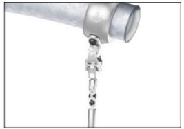
The swing hangers are made of stainless steel brackets and can move over two axis. The flange bearings are silicone enriched to make the suspension maintenance free. The connection to the rope is made with stainless steel chain.
