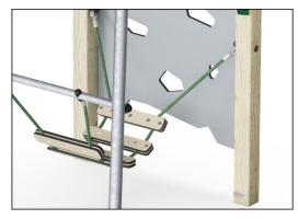
Corocord ropes of UV-stabilized PES rope strands with inner steel cable reinforcement. The polyester yarn is made from +95% postconsumer materials and is inductively melted onto each strand. PES has high strength with excellent resistance to abrasion and UV radiation. The hammock boards are made of EcoCore HDPE material made from +95% Postconsumer materials.
