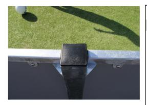
The posts are made of  $80 \times 80 \times 3$ mm profile with horizontally, 6mm welded flanges. This will enable an easy installation and strong construction. The low-density polyethylene post caps are attached with blind rivets.
