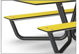
All boards are made of High Pressure Laminate HPL with a .7 in. thickness according to EN 438-6 and has a nonskid surface texture. The multilayer construction makes the boards durable and suited for outdoor use, with a high resistance to impacts, scratches, fire, water and humidity, as well as high UV stability.
