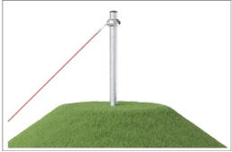
Corocord ropes with 19mm+ diameter are known as a 'Hercules' rope type which is formed from galvanised six-stranded steel wires. Each strand is tightly wrapped with PES yarn, which is melted onto each individual strand. Ropes are highly wear-and vandalism-resistant and can be easily replaced on-site if needed. The steel surfaces are hot-dip galvanised inside and outside with lead-free zinc. The galvanisation has excellent corrosion resistance in outside environments and requires low maintenance.
