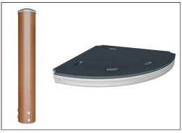
ELEMENTS decks are made of 17.8mm thick HPL supported by a uniquely designed aluminium frame with multiple attachment options by the usage of aluminium connectors. The main posts are made of high-quality pregalvanised steel with a powder-coated top finish. Post tops are closed with caps of UV stabilised nylon (PA6).
