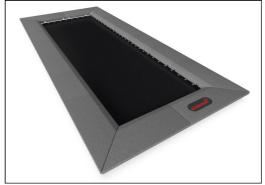
The tiles are moulded in grey granulated recycled rubber (SBR/NR), and the KOMPAN logo is made from EPDM Ethylene Propylene Diene Monomer. Inside each of the rubber tiles, there is a 3 mm hot-dip galvanised steel plate.
