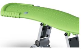
Starsurfer is made of medium density PE with excellent impact strength and usable within a large temperature span. Hollow plastic components are made of 100% recyclable PE made from 33% post-consumer materials. Molded in one piece with minimum 5mm wall thickness. The textured surface provides a slip resistant surface for safe play.
