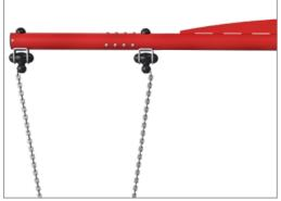
The seat hangers are made of high quality UVstabilized nylon (PA6) housing with integrated lifetime sealed ball bearings. The chains are fixed by a stainless steel hook with theft proof snake-eye bolt in a turn able anti twist housing.
