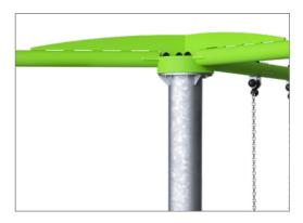
Center post is hot-dip galvanized in dimension  $\emptyset$ 159 x 4 mm. Horizontal beams are hot-dip galvanized and powder coated in dimension  $\emptyset$ 76,1 x 3,6 mm.
