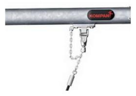
KOMPAN heavy duty designed swing hangers of stainless steel with anti-twist function. The hangers are attached to the cross beam on a welded bracket with two bolts, The bearings are embedded with silicone lubricant and needs no further lubrication.
