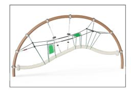
The bent arches are holding the tensioned net structure without additional disturbing fasteners. Therefore, the arches are produced from high degree stainless steel to allow movement of the net on the surface of the steel arches. The surface is then treated to create a shiny finish.
