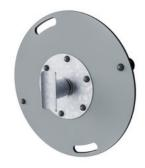
The bearing house is made from hot dip galvanised steel. The bearing shaft is made from stainless steel AlSI304. The bearing itself is made from Polyoxymethylene (POM), an engineering thermoplastic with a high stiffness, low friction, and excellent dimensional stability.
