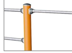
All bars intended for pull ups are made of solid, ø32mm x 138 m, hot dip galvanized, S235JR steel bars. This diameter gives the right grip for everyone.
