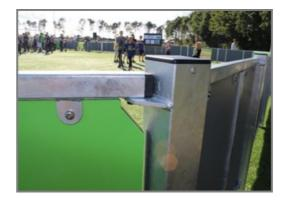
The HDPE panels are connected with M8 stainless steel bolts to 42.5 x 40 x 3mm welded flanges. These connections are not visible from the inside and create a strong and safe connection.
