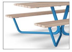
Galvanisation is manufactured with a two-step process which includes light grinding and clean sweeping, which is then finished with a top powder coating to 70-120 µm thickness.
