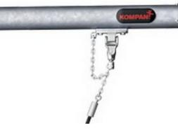
Upper chain and safety chain are made of highquality stainless steel to guarantee the durability of the product. KOMPAN's swing hangers are heavy-duty and designed with stainless steel and anti-twist functions. The hangers attach to the cross beam on a welded bracket with two bolts. The bearings are embedded with silicone lubricant and need no further lubrication; ensuring low maintenance.
