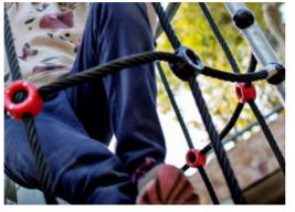
Ropes of UV-stabilized PES rope strands with inner steel cable reinforcement. The polyester yarn is made from +95% post-consumer materials and is inductively melted onto each strand. KOMPAN GreenLine versions are designed with ultimate environmentally friendly materials with lowest possible CO2e emission factor. TexMade post, EcoCoreTM panels of 95% post-consumer recycled waste and molded PP decks.
