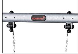
The swing hangers are made of high quality UVstabalized nylon (PA6) housing with integrated lifetime sealed ball bearings. The height adjustable chains are fixed by a stainless steel hook with theft proof snake-eye bolt in a turn able anti twist housing. All seats with two chain fixation are available with either standard or anti-wrap suspension.
