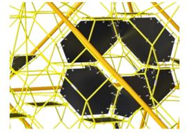
Corocord membranes consist of friction-proof rubberised material of conveyor belt quality with excellent UV resistance. Tested and compliant with REACH requirements for PAH. Embedded is a four-layered armouring made of woven polyester. The armouring and the two surface layers result in a total thickness of 7.5 mm.
