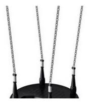
KOMPAN designed curved toddler seat is made The double steel yoke suspension provides the with an insert of 21.25 mm thick plywood from unique parallel movement of the seat. The swing hangers are made of high quality UV stabilized molded in UV stabilized PUR which retains its nylon (PA6) housing with integrated lifetime properties in the temperature range of -30°C to sealed ball bearings. The height adjustable chains are fixed by a stainless steel hook with
