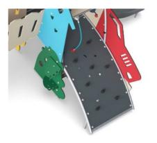
The curved climbing wall is made of Ekogrip® panel that consists of a 15mm thick PE base with 3 mm top-layer of soft rubber with a non-skid effect.
