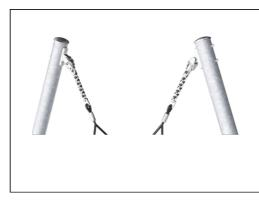
The swing hangers are made of stainless steel brackets and can move over two axis. The flange bearings are silicone enriched to make the suspension maintenance free. The connection to the rope is made with stainless steel chain.
