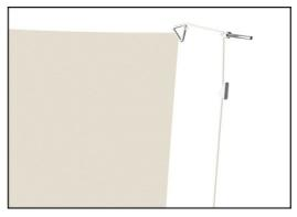
All fixation points are equipped with steel brackets to ensure strong connection to the nylon rope used for tightening.
