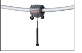
The hang-on puller is designed with a welded steel core and covered with low-density PE housing. The two hot-dip galvanised steel handles are angled to provide the best possible ergonomic while gliding. The wheels of the puller are made of low noise TPU and installed with sealed ball bearings. The Robinia products come in a number of standard colour options. The wood can also be supplied as untreated or with brown painted with a pigment that maintains the wood colour.
