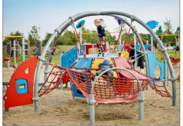
The steel arches are hot-dip galvanised inside and outside with lead free zinc. The galvanisation has excellent corrosion resistance in outside environments and requires low maintenance.
