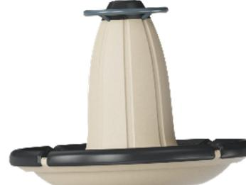
The central part of the Boogie Spinner is made of recyclable polyethylene (PE) made from 33% post consumer materials and is rotomolded in one piece with integrated metal thread bushings and water drain holes to ensure high durability in all climates around the world.
