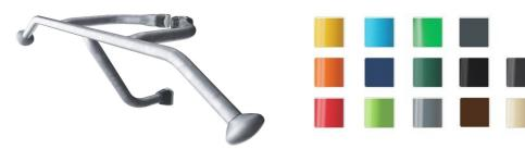
The frame of the leg lift is made from Ø38 x 2mm HDG steel tube. The support plates are made from 15mm Ekogrip®, a 15 mm PE plate with a 3 mm top-layer of thermoplastic rubber with non-skid effect. The arm supports are 110 x 195mm, 580mm apart, and 1315mm above ground. The back support is 335 x 500mm. The opening in the back is 30 x 350mm. The pull up bar is made from Ø32 mm HDG steel bar. The bar is 1080mm wide and 2300mm above ground
