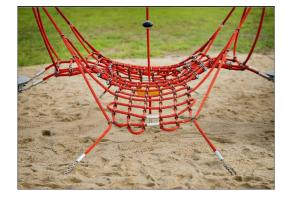
Ropes of UV-stabilized PES rope strands with inner steel cable reinforcement. The polyester varn is made of +95% Post-consumer materials and is inductively melted onto each strand to obtain excellent wear and tear resistance.
