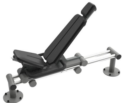
The seat and head support are made of Polyurethane Rubber and have a steel insert plate that connects it to the steel frame. The seat is adjustable in 14 different settings to fit users from 140/ 205 cm tall and to vary the type of exercises. The seat is positioned under a 12-degree angle and the back supports a 48-degree angle. The back support has a groove, accommodating a comfortable position.
