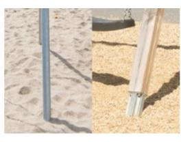
The post of the A-Frame swings are available for surface anchoring with expansion bolts or inground in 60cm or 90cm depth. The hot dip galvanised steel legs are anchored directly in the ground. Pine wood posts are elevated from ground by a unique profiled hot dip galvanised steel footing.
