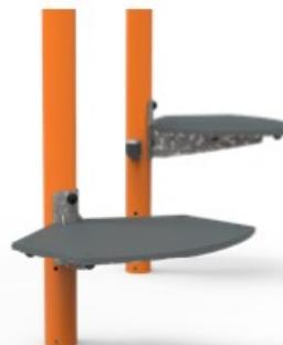
The top plate for the jumping platform is made of Ekogrip® panels that consist of a 15 mm polyethylene bottom layer, with a 3 mm top-layer of thermoplastic rubber with a non-skid effect for safe jumping exercises under all-weather circumstances.
