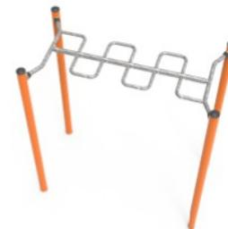
The snake ladder is made of hot-dip galvanized s235 steel with the following dimensions Ø38 x 4mm. The steel surfaces are hot dip galvanised inside and outside with lead free zinc. The galvanisation has excellent corrosion resistance in outside environments and requires low maintenance.
