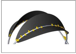
Steel frame supports Ekogrip® panel to form the roof. The Ekogrip® panel consists of a 15mm thick PE base with 3 mm top-layer of rubber.
