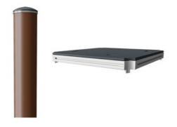
ELEMENTS decks are made of 17.8mm thick HPL supported by a unique designed aluminium frame with multiple attachment options by usage t= 2mm. of aluminium connectors. The main posts are made of high quality pre-galvanized steel with powder coated top finish. Post tops are closed with caps of UV stabilized nylon (PA6).
