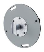
The bearing house is made from hot dip galvanised steel. The bearing shaft is made from stainless steel AISI304. The bearing itself is made from Polyoxymethylene (POM), an engineering thermoplastic with a high stiffness, low friction, and excellent dimensional stability.
