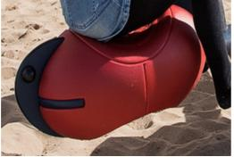
The seat is made of recyclable PE and moulded in one piece with a minimum 5mm wall thickness. PE has high impact resistance across a wide temperature span which ensures vandal resistance in all locations.
