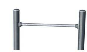
Steel posts are galvanised inside and outside with powder coated top finish. This provides an ultimate corrosion resistance in all climates around the world. The turnbars are hot dip galvanised inside and outside with lead free zinc. The galvanisation has excellent corrosion resistance in outside environments and it requires low maintenance.
