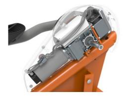
The Innovative self-powered electrical motor and gear providing a virtual flywheel to give real road experience. The resistance works as and automatic drive and adapts automatically. The users can overwrite the automatic drive manually by changing the resistance in 10 steps (45-750 Watts) through the App or screen.
