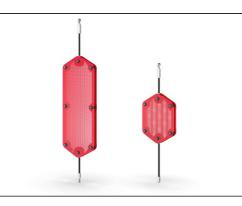
Turnable optic panels of two 7mm thick polycarbonate plates with a distance of 40mm. The inside graphic print consist of an inner image layer and outer transparent protection layer. Both PC panel and the water-based lacquer are UV stabilized to prevent fading of the print.
