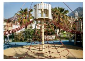
Corocord 16mm ropes are special 'Hercules'-type with galvanized four-stranded steel wires and a steel wire core. Each strand is tightly wrapped with PES yarn, which is melted onto each individual strand. The ropes are highly wear-and vandalism-resistant and can be replaced at site if needed.
