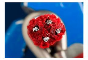
Corocord 16mm ropes are special 'Hercules'type with galvanized four-stranded steel wires and a steel wire core. Each strand is tightly wrapped with PES yarn, which is melted onto each individual strand. The ropes are highly wear-and vandalism-resistant and can be replaced at site if needed.
