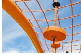
Fully colored EPDM rubber discs with smooth surface. The moulded EPDM surrounds a hot dip galvanized steel core that ensures both the stability of the discs and durable fixation to the rope.
