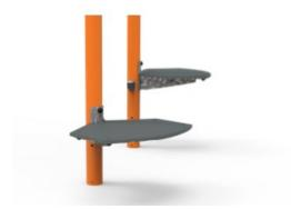
The top plate for the jumping platform is made of Ekogrip® panels that consist of a 15 mm polyethylene bottom layer, with a 3 mm top-layer of thermoplastic rubber with a non-skid effect for safe jumping exercises under all-weather circumstances.
