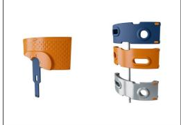
The climbing elements displayed are moulded in one piece with a minimum 5mm wall thickness. The climbing elements are made of recycable PE which has a high impact resistance across a wide temperature span which ensures vandal resistance in all locations.
