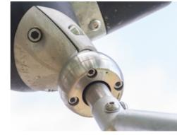
Bearing systems in heavy duty design in a maintenance free construction. All steel bearings are fully closed and lifetime lubricated.
