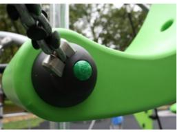
Larger activities are made of 100% recyclable PE. The play shell displayed is molded in one piece with a minimum 5mm wall thickness. PE has high impact resistance across a wide temperature span which ensures vandal resistance in all locations.
