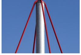
In the centre of the net is the mast, made of high quality seamless steel. The structure of the mast as an oscillating support is statically favourable and equalizes the oscillations in the net. The masts are hot dip galvanised as standard, with the design option of additional powder coating.
